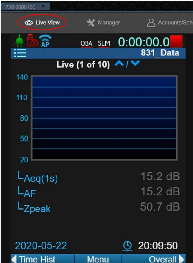
The Live View appears differently for each instrument. *Figure 1-6* shows the SoundAdvisor 831C Live View as an example.
