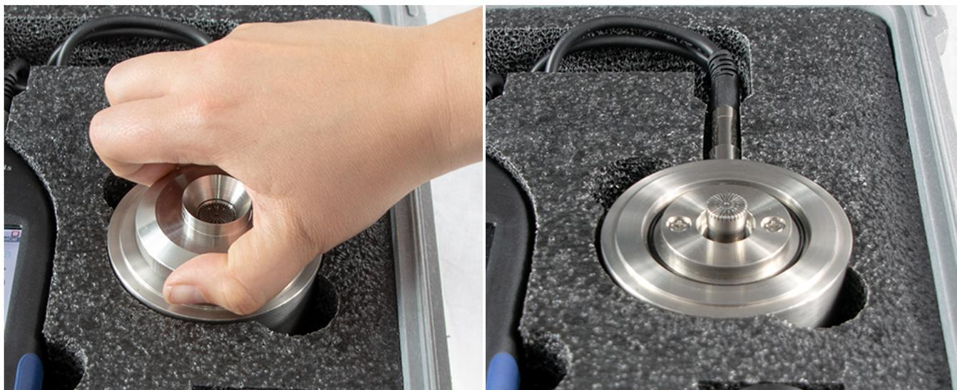
**Step 5** Carefully mount the calibrator over the microphone, using an adapter for a 1/2" mic (ADP019).
