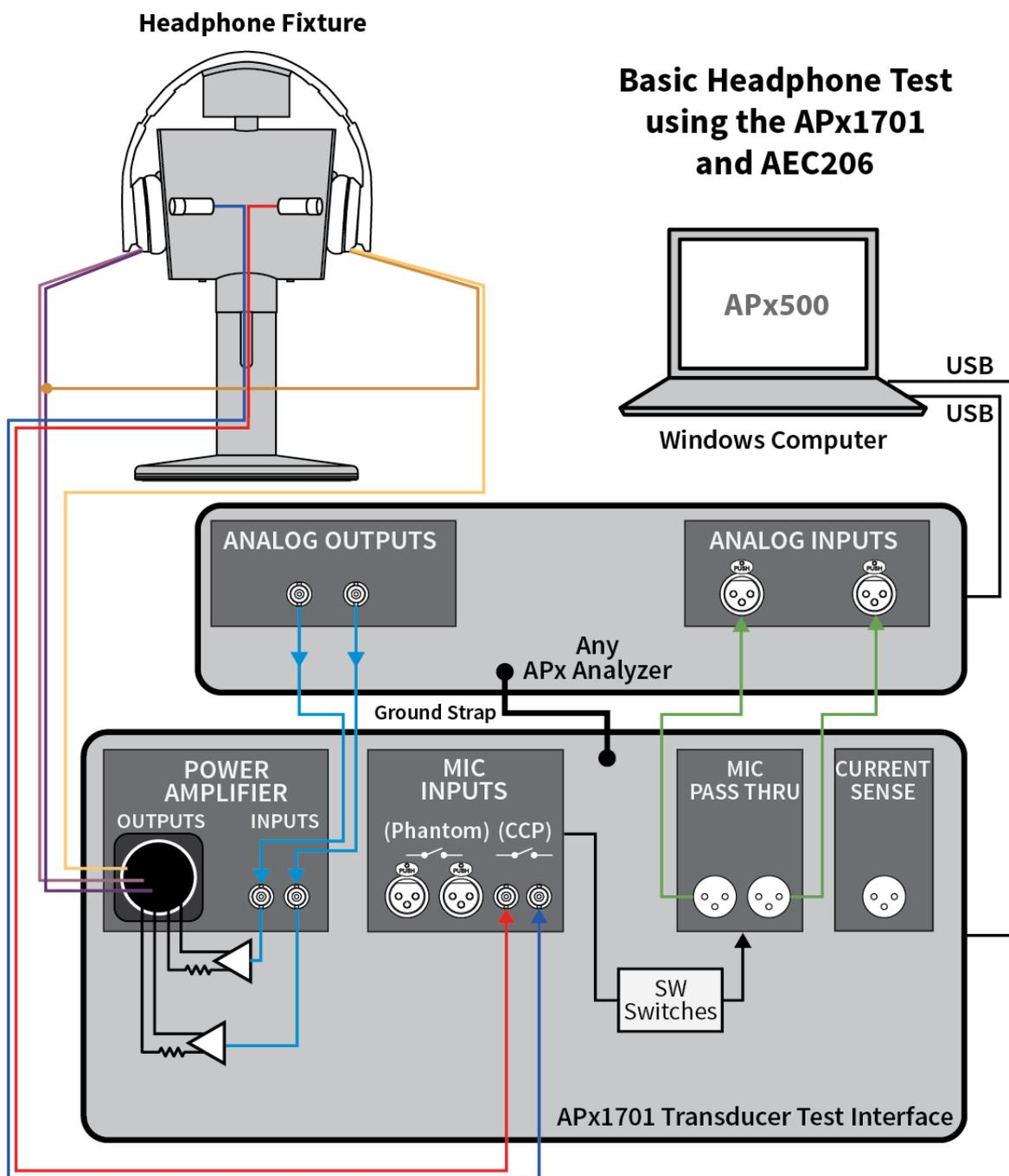
FIGURE 1-5 Headphone Test with Impedance/T-S
