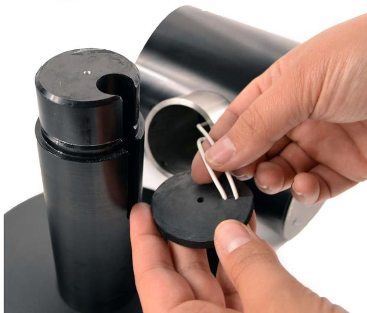
**TAKE NOTE** Align the gasket slit with the center of the cavity in the neck, so the cables run down into the neck.
