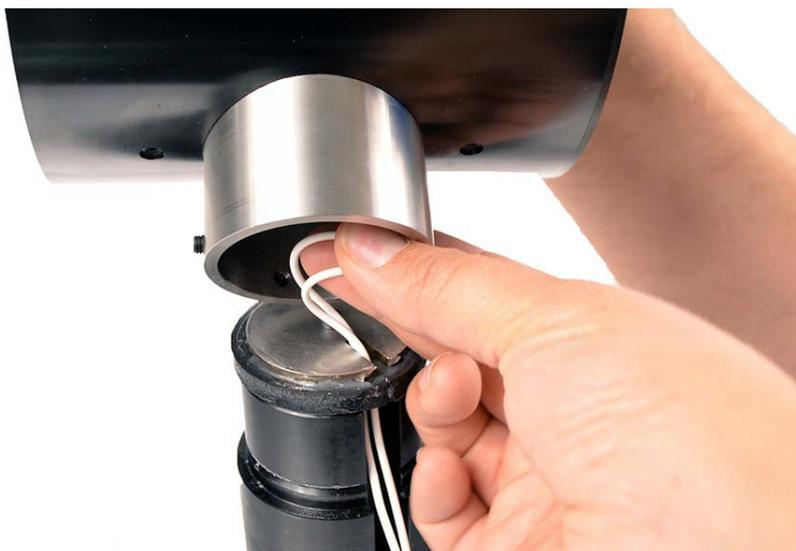
**Step 10** With the head vertically aligned with the neck, mount the head onto the neck. You will feel resistance and a pressure build up in the head, this is normal.
