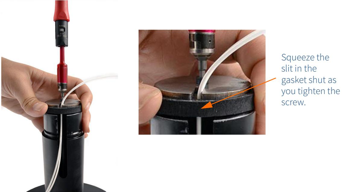
**FIGURE 2-15 Grease gasket**
