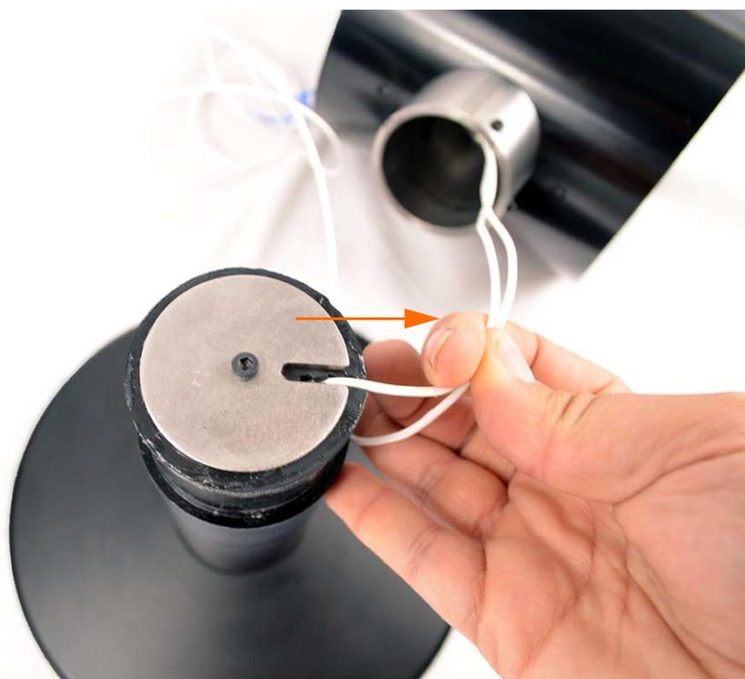
**Step 7** Gently pull the AEC304 completely out of the head. Feed the cable up through the head and out the side.
