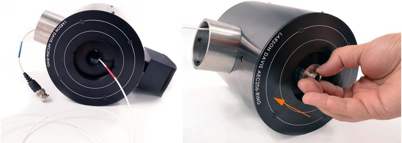
**Step 3** Using the 2.5 mm hex driver, unscrew the washer/gasket screw completely. Pull off assembly, and then separate the washer from the gasket.
