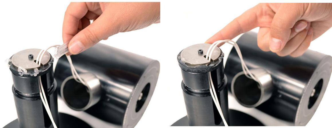
**Step 9** Feed the slack of the cables into the head. Ensure all cables are all the way in before moving on to the next step, if the
