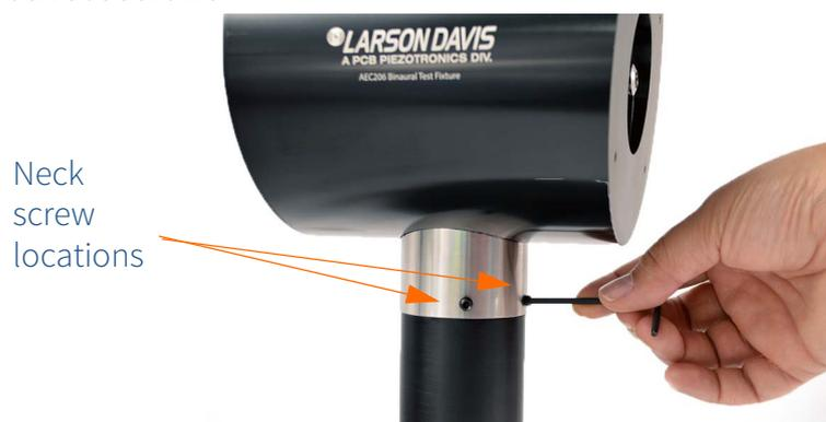
**Step 5** Hold the base down with one hand and pull from the hat to separate the head and the neck. There is a vacuum seal to the head and the neck, additional force may need to be applied to the base, however avoid twisting, this may cause the cables to break. Set head next to the stand with the cables loose.
