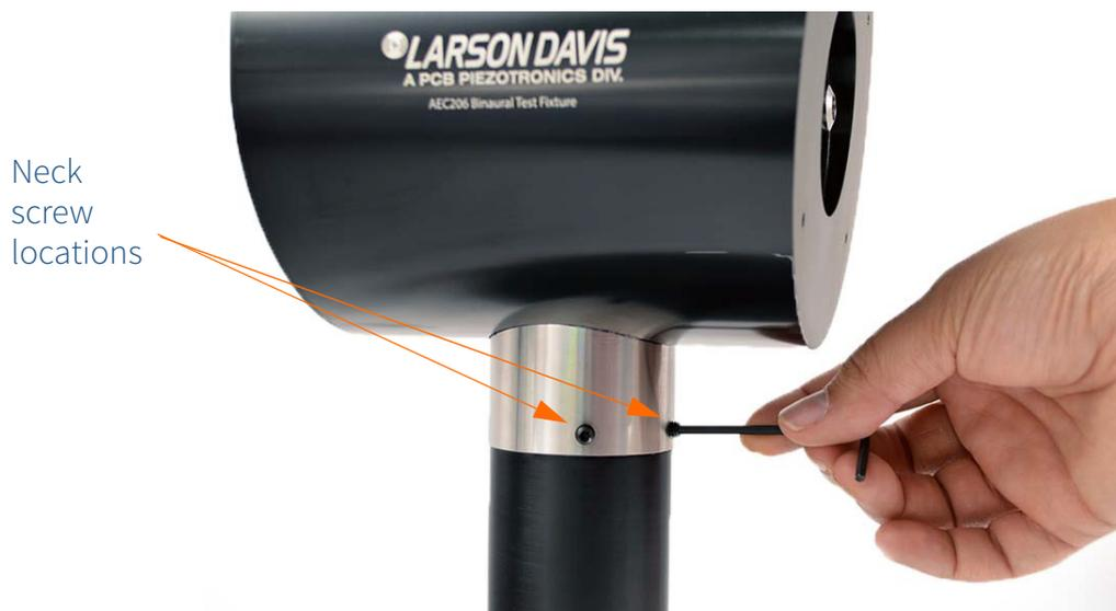
**Step 12** Ensure the AEC304 is completely pushed into the head. Using a torque screwdriver set to 40 oz-in, turn the set screws on the head until push rod is clamped.
