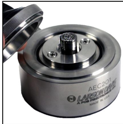
**FIGURE 3-1 Coupler being installed on AEC201**
