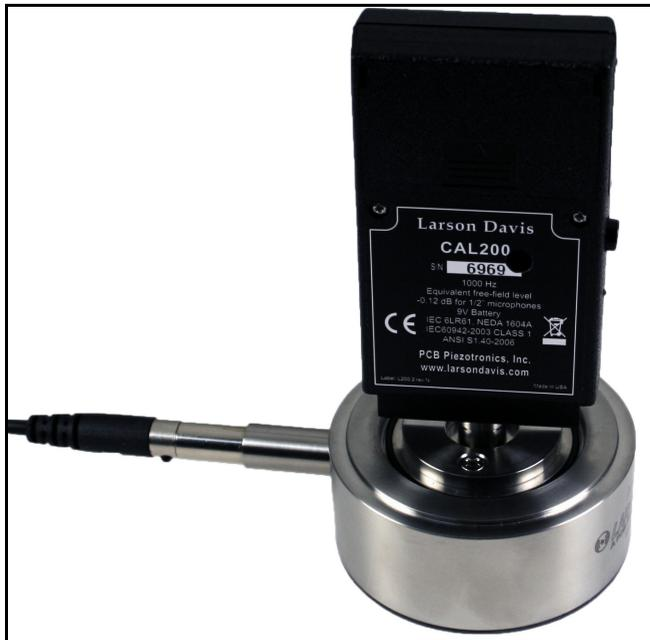
**FIGURE 2-5 CAL200 being activated on AEC201**
