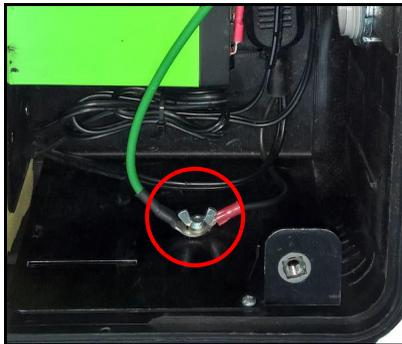
**FIGURE C-7** Connected Ground
