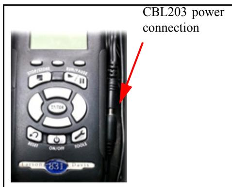
**FIGURE C-6 Connected Power**
