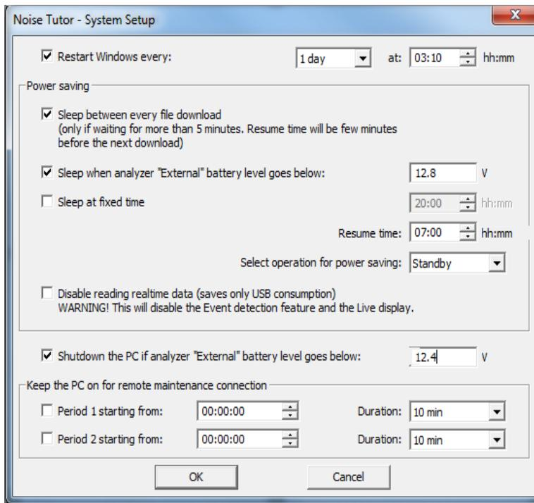
**FIGURE 3-11 Power Saving Setup**
