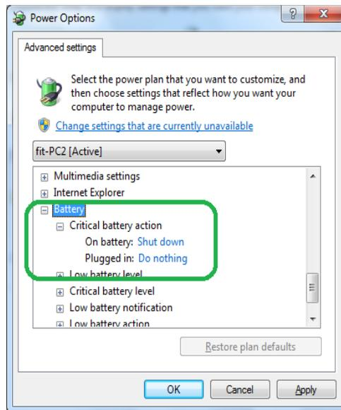
**FIGURE 3-7** Critical Battery Action Settings
