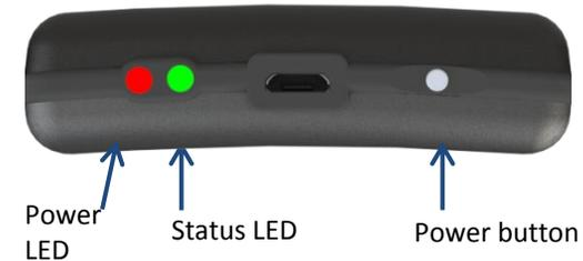
To check meter operation, refer to the Power and Status LEDs.
