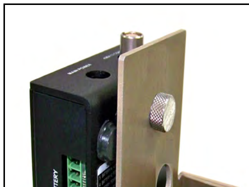
FIGURE 2-14 Mounting of 831-INT
