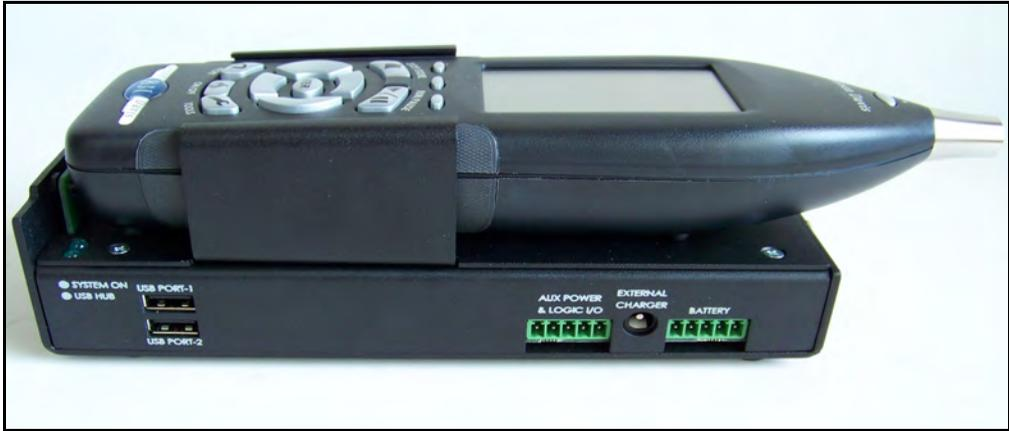
**FIGURE 2-2 831-INT with Model 831: Right Side View**
