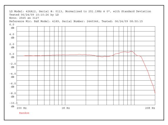
FIGURE A-14 426A12 with 2565 Microphone: Random Incidence
