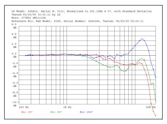
FIGURE A-3 426A12 with 377B02 Microphone: 30, 90 and 150 degrees
