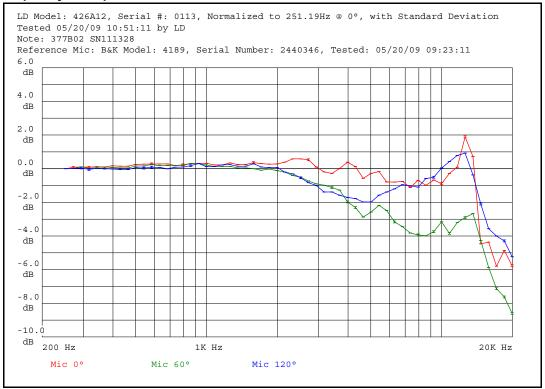
FIGURE A-1 426A12 with 377B02 Microphone: 0, 60 and 120 degrees
