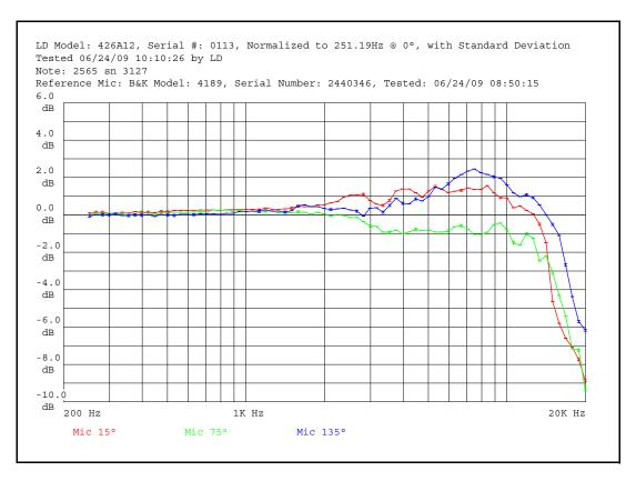
FIGURE A-11 426A12 with 2565 Microphone: 15, 75 and 135 degrees
