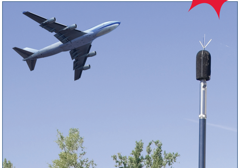
Typical Model 426A12-FF airport noise monitoring installation.
