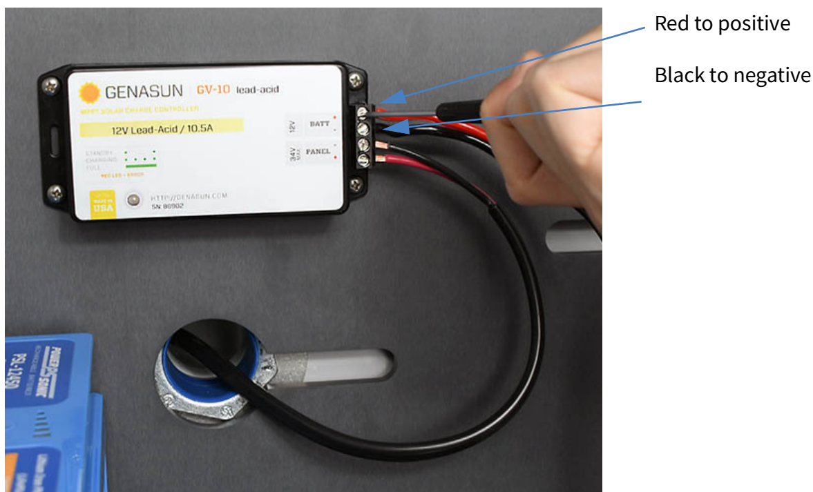
FIGURE 4-13 CBL226-03 to Solar Charger
