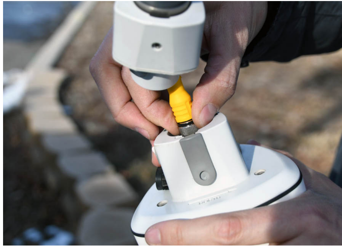
FIGURE 4-17 Feed CBL229-20 Through Weather Arm
