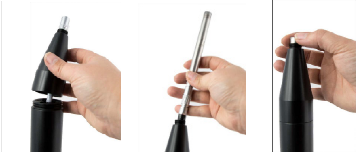
FIGURE 2-3 Replacing the top cap and preamplifier
