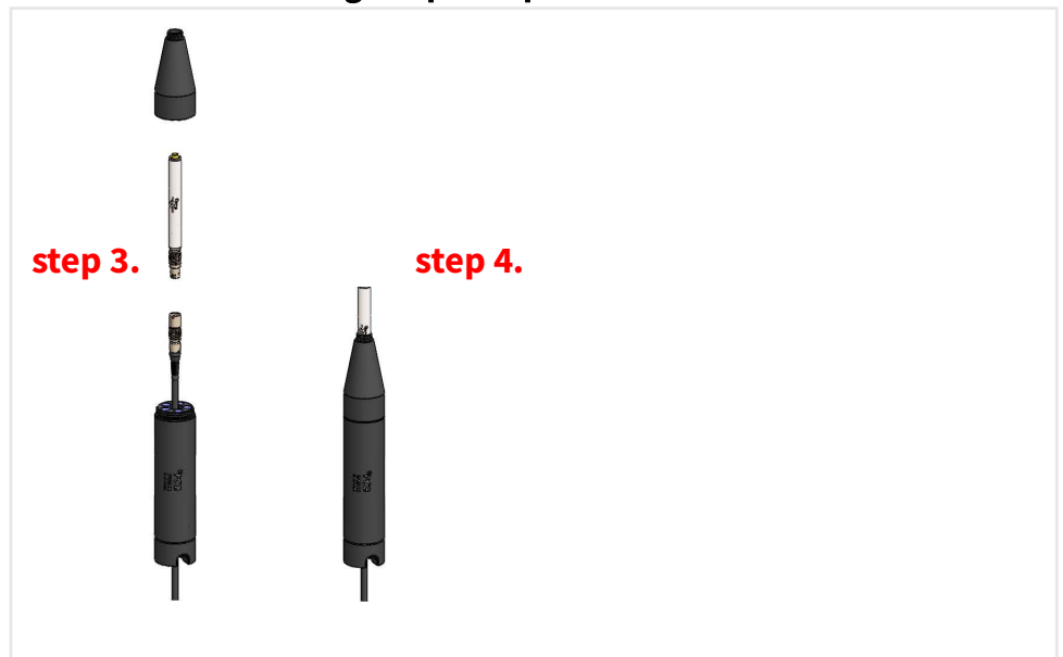
FIGURE 1-4 Connecting the preamp
