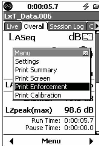
Step 5. Tear off the Measurement and Calibration printouts and complete by writing the location in the space provided and signing the printouts.
