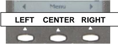
These three buttons allow you to control the views and functions available on the LCD display. They are used as both FUNCTION
