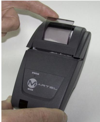
roll of paper, hold about 5cm of paper outside the printer as the roll is dropped into the paper reservoir. Close the lid by applying equal amounts of pressure on each side until the lid is locked into position.
