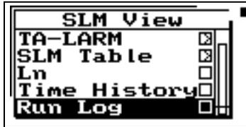
Press the right arrow key or the Check Key to view the Run Log display. The display is shown below:
