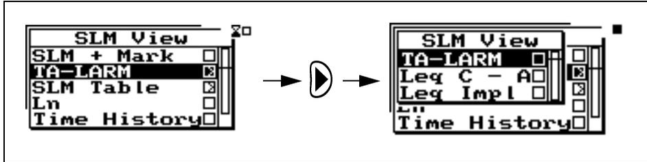
Press the right  $\blacktriangleright$  arrow key or the Check  $\checkmark$  Key to view the TA-LARM displays. The displays are shown below:
