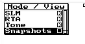
Highlight “Snapshots” and press the Check (✓) key to access the snapshot data.
