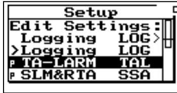
Press the Check
