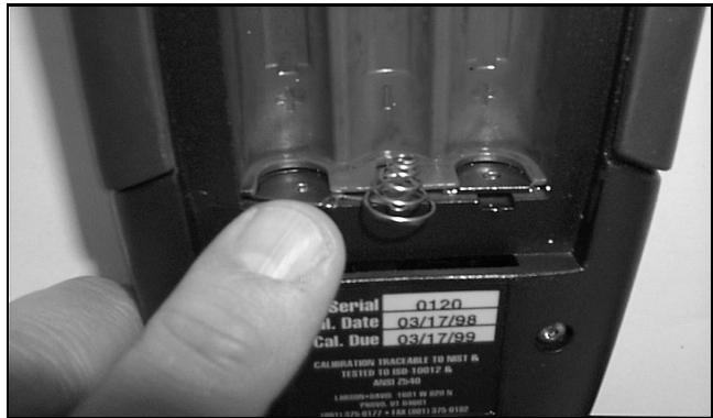
Figure 1-8 Battery Terminal Assembly orientation.
