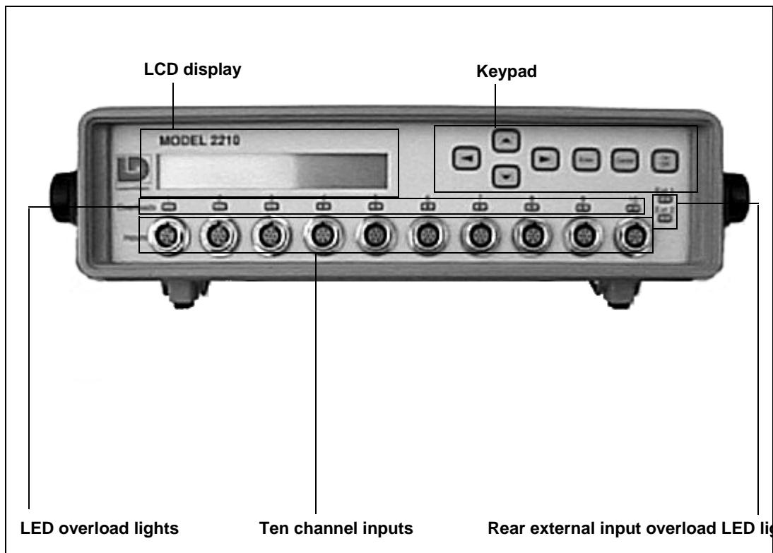
Figure 2-1 *Model 2210 Front Panel.*
