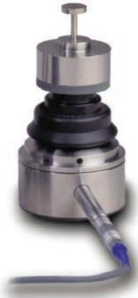
The AEC100 Coupler is a precision acoustic coupler designed primarily for the calibration and test of supra-aural earphones used in audiometry. It allows accurate and repeatable measurements within its frequency response (up to 8 kHz). It may also be used for production testing where correlation between the coupler and real ear response is not a requisite.
