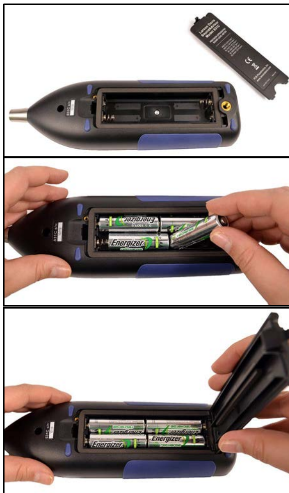
FIGURE 2-3 Installing batteries into the 831C.
