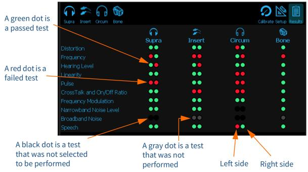
Clicking (or tapping) on a dot will jump you to that portion of the test suite. This is so you can rerun any failures, run tests that were missed, or quickly view results.
