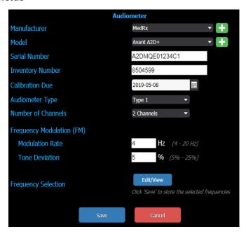
Step 7 Select Edit/View button for the Frequency Selection. You can select high, low, set to default, or manually select and deselect values. These are frequencies that will be tested. When finished, Continue and it will return you to the Audiometer screen.
