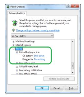
FIGURE 3-7 Critical Battery Action Settings
