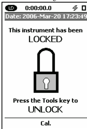
FIGURE 21-14 Locked with Calibration Permitted
