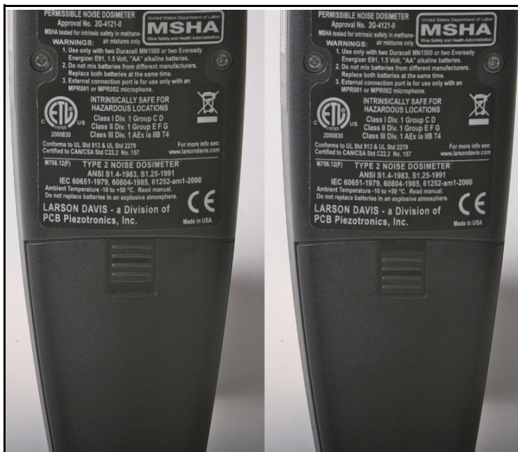
FIGURE 1-7 Moving the battery door sliding tab
