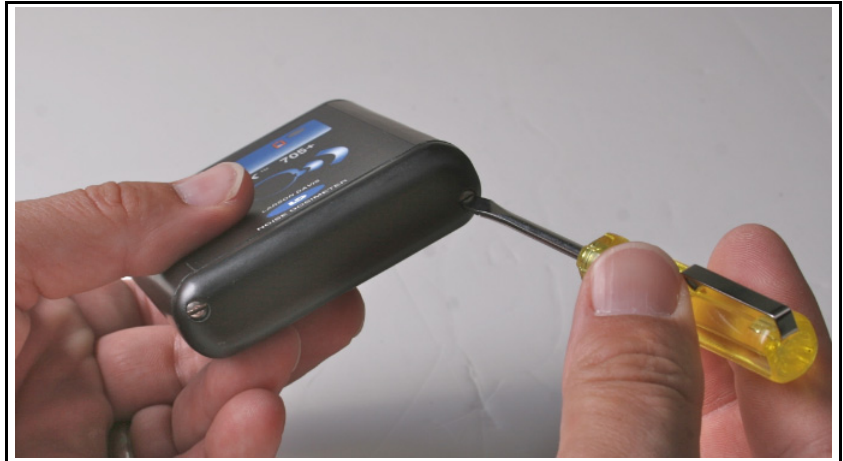
FIGURE 1-11 Removing the battery door
