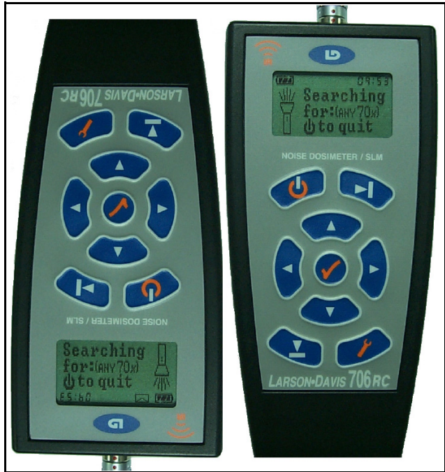
FIGURE 3-1 Inverted and Standard Display Modes
