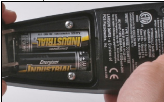
FIGURE 1-9 Re-inserting the battery door
