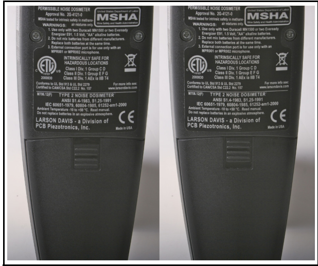
FIGURE 1-10 Locking the battery door
