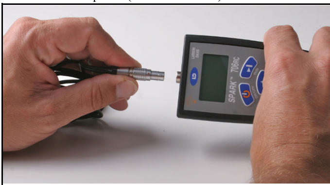
FIGURE 1-4 Aligning the microphone connectors
