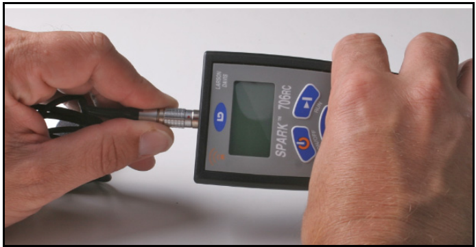
FIGURE 1-5 Connecting the microphone
