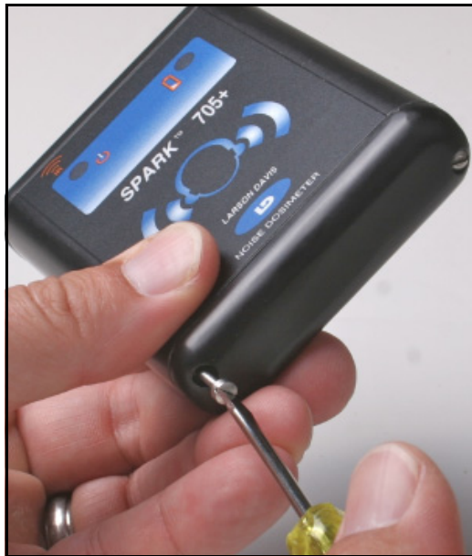
FIGURE 1-14 Replacing the battery door
