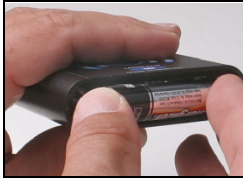
FIGURE 1-13 Replacing the battery
