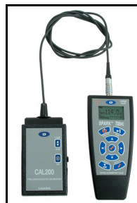
FIGURE 2-15 Calibrating the Spark™
